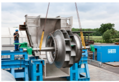
Figure 4 and 5: M-Series fan in large-scale testing facility
